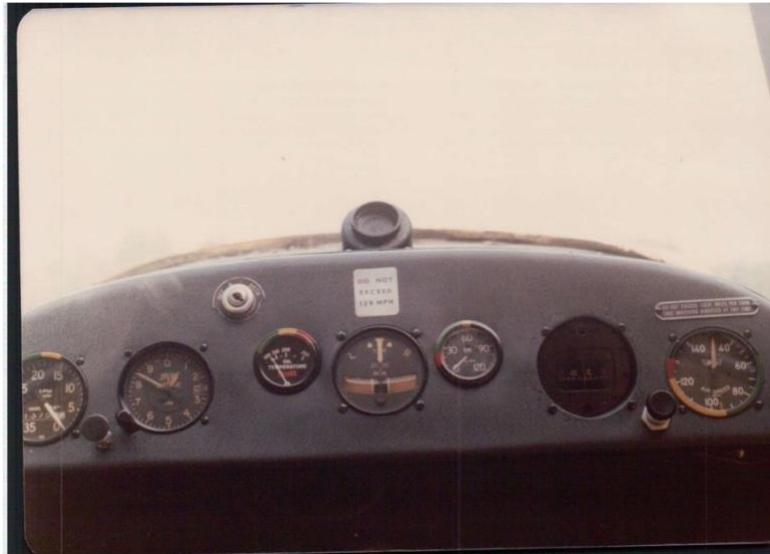
The Champs control panel with the (leaky) Model A gage location on top of the panel (Courtesy of Charlie Hensley)
